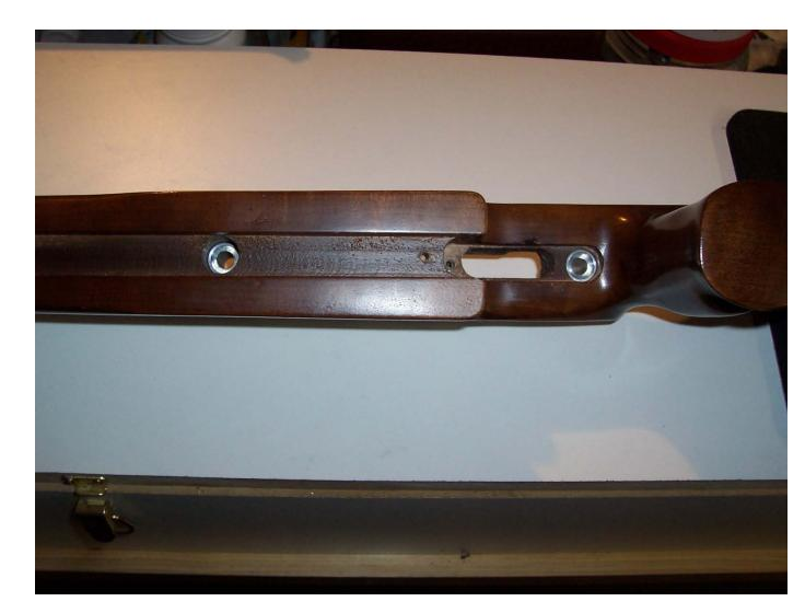
Stock milled to accept pillars and pillars glued into the stock with action aligned and pillars bolted to action. After pillar bedded, I glass bedded the stock -with Acraglas<sup>®</sup>. I then milled out the stock to accept the magazine and the new trigger (not shown).
