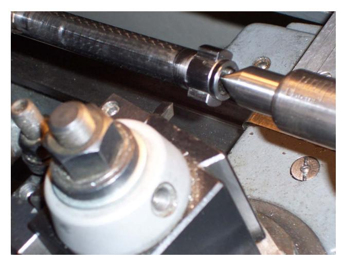
After I turned the bolt face, and both sides of the bolt lugs, I lapped them into to the action to ensure that there was a 100% lug fit with the action shoulders. They look real good after lapping. The new headspace is 0.950". I am now on to turning the shank, threading, insetting, and chambering the barrel.
