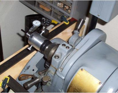
Barrel Setup for Bench-rest Quality Chambering – setups take longer than the actual turning
