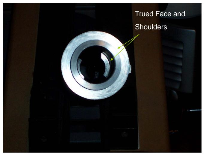
Removed .003" from action face and .002 from shoulders. Action sides remain untouched. Action is now ready for lapping in the lugs once the bolt lugs are trued up. I use anti-seize compound to verify 100% lug engagement.
