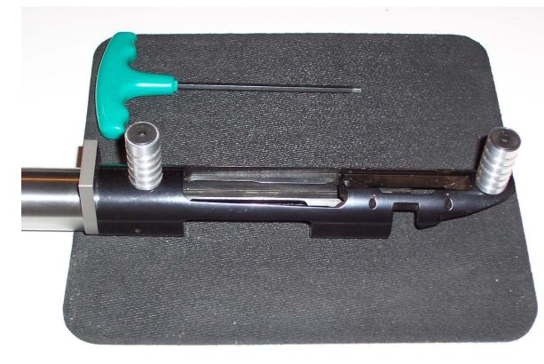
Made pillars and bolts to fit the action and stock to provide on metal to metal action insertion. Special flat head bolts were made to ensure accurate action lockup in the stock.
