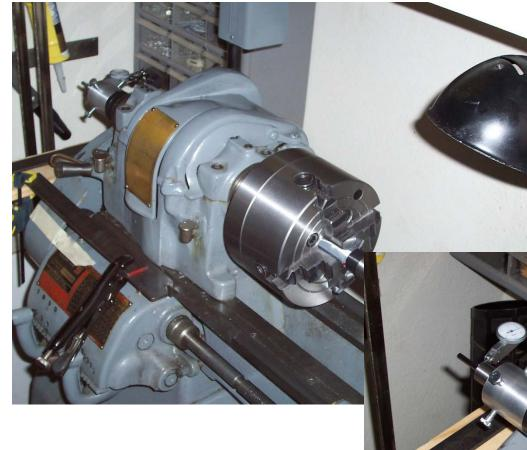
I try to get the bore run-out within .0001" at both ends of the barrel and check to make sure I'm not stressing or bending the barrel in any way by using an o-ring on the spider – the electrical tape holds it in place so spider will flex if barrel is stressed.
