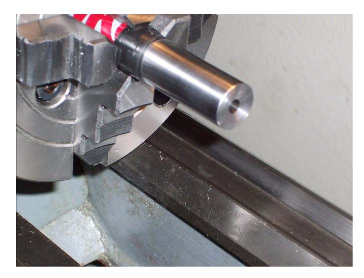
I use a cotton swab to ensure that no burs were caused when cutting the crown. A little cleanup and this barrel is now ready for installation.
