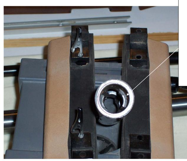
You can see that the shoulder on the right has been bearing most of the bolt lug load. This will need to be fixed to improve accuracy of this gun.
