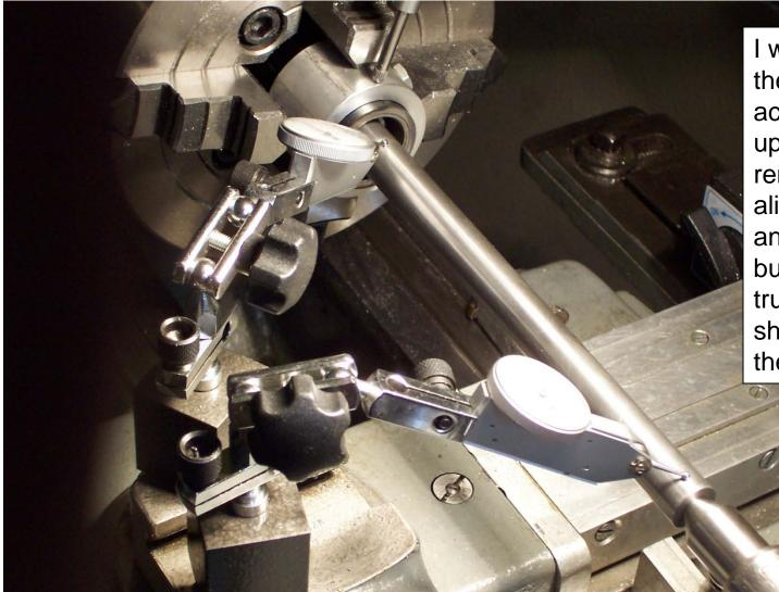
I will now turn the face of the action to true it up then I will remove the alignment rod and the taper'd bushings and true up the shoulders inside the action.
